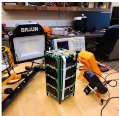
The completed 2U CubeSat Jagsat-1 being tested for solar panel and power system performance before delivery to NanoRacks in Houston.
