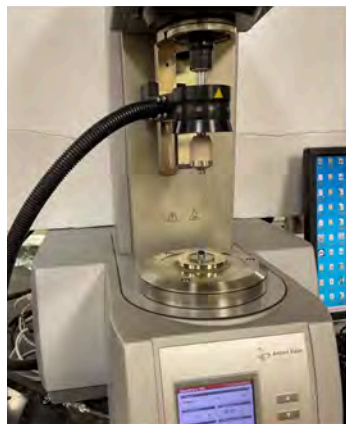
Dynamic Shear Rheometer (DSR) set-up for asphalt binders' various performance characterizations.
